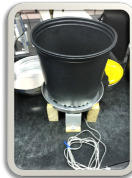
Fig. 5a and 5b. Tipping gauge beneath container for micro-irrigation (left, 5a) and for sprinkler irrigation (right, 5b). Medical wrap was placed around pizza pan to inhibit sprinkler irrigation from entering pan.
