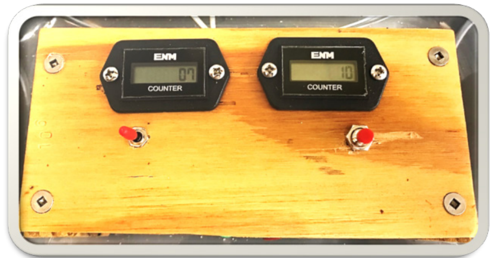
Fig. 4. Digital counters were connected to gauges, and both were energized with 9-volt battery.
